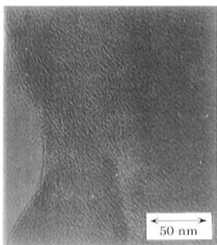
Figure 4. TEM photograph of PVA-alumina hydrate film.
